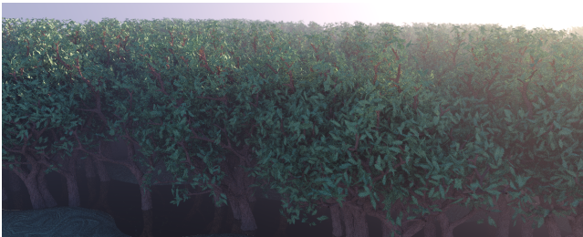
Figure 7: Stress test: this forest consists of two million patches, which would need a triangle mesh equivalent of more than 1050 billion triangles if fully tessellated. Fully path traced with motion blur, the image renders at 1920 \times 768 \times 16 samples in 2:24 minutes on a four core machine.
